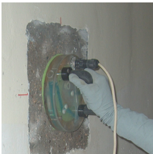
Fig. 8. Arrangement used for PVT and corrosion rate measurements.
